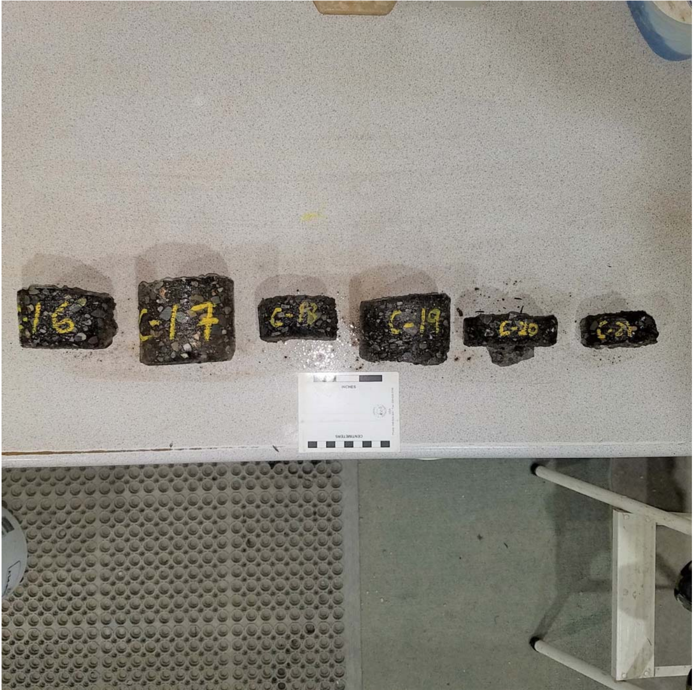
Photo M: Photo of asphalt cores C-16 to C-21 from left to right. Scale in inches and centimeters.
